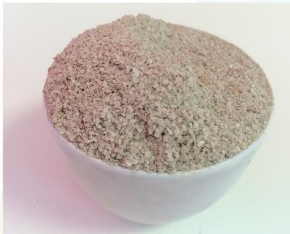
Picture 3: Struvite obtained at Calahorra WWTP
