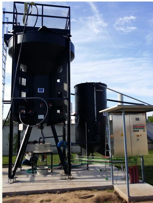
Picture 1: Crystallization reactor
